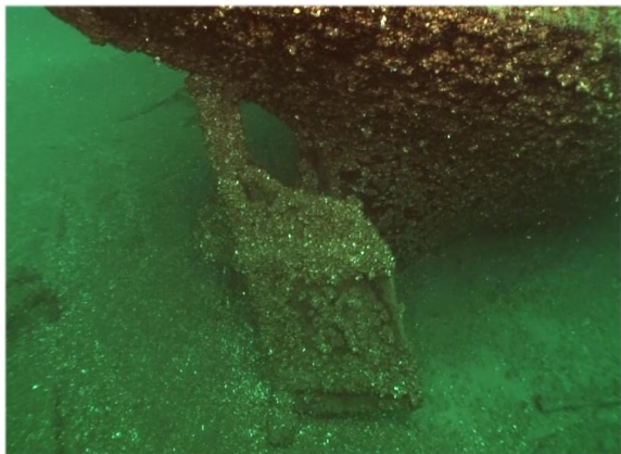
The rudder is locked in a position to make a hard starboard turn
