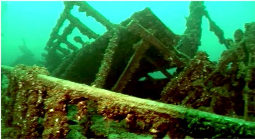
Much of the superstructure above the main deck has collapsed
