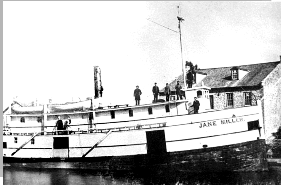
The Jane Miller was a stubby and narrow vessel designed as a “coaster” to service the small communities and lumber camps of Georgian Bay.
