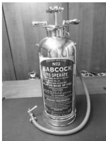
Babcock Fire Extinguishers were filled with water, dry acid, and bicarbonate of soda. When sealed the pressure inside could shoot water 50 feet
